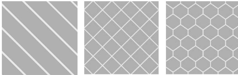
Figure 4: General internal filling patterns on 3D Printing
