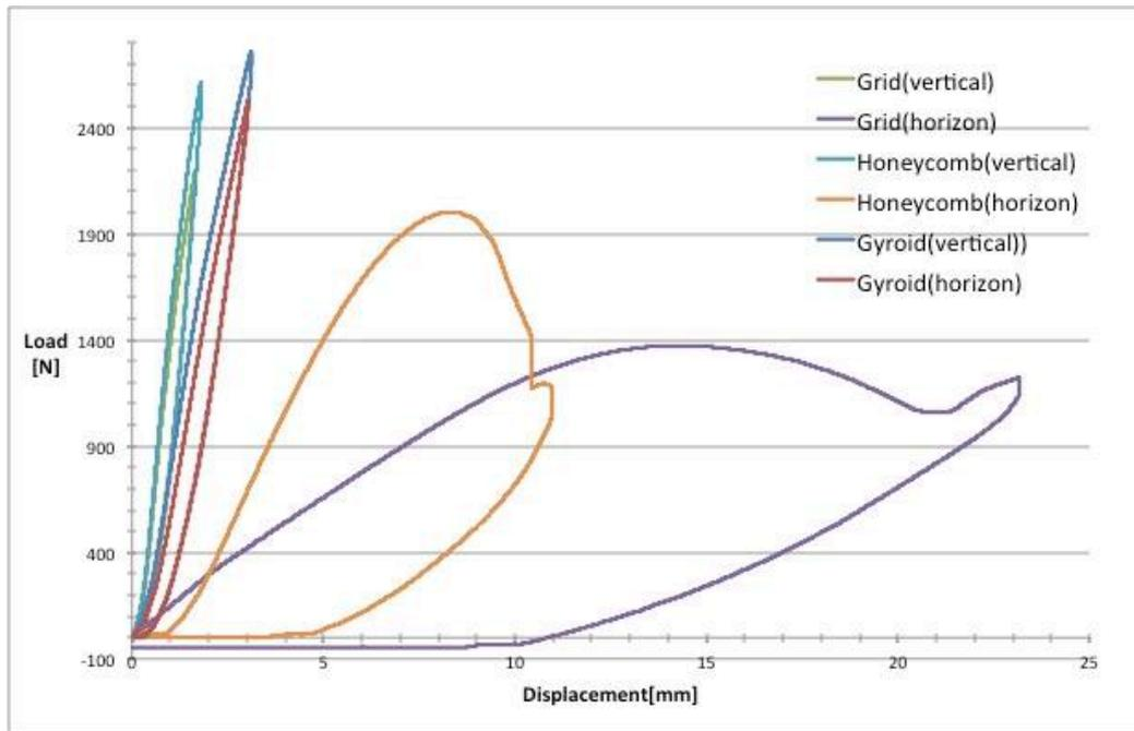
Figure 7: Structural mechanical properties of each Internal filling pattern
