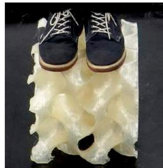
Figure 6: Gyroid Structure Module
